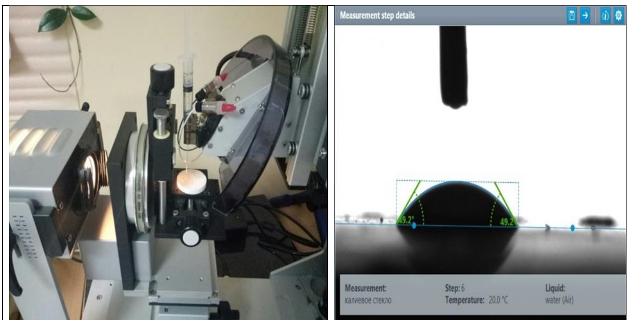
Figure 2 - KRUSS DSA30 contact angle measuring device
